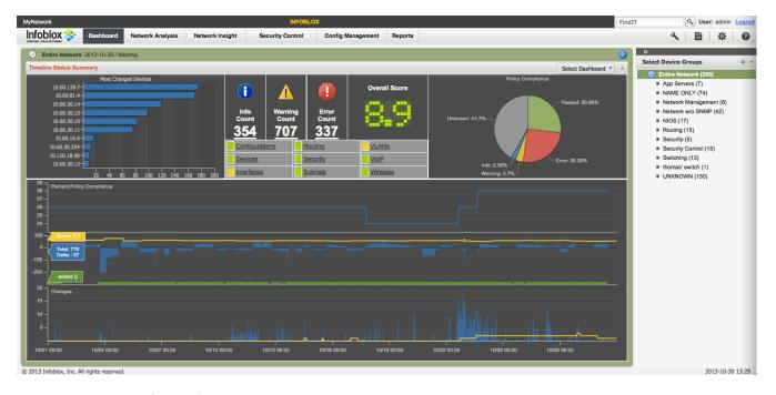
This is the Timeline Status Summary. You can see the devices with the most changes over the past month in the upper left corner of the screen. Depending upon the location and use of these devices, this could be a normal or abnormal. You can click on the individual graph to drill down for details on the changes. The change graph on the bottom of the screen shows when changes occurred. This allows you to determine if the spike in changes correlates to a network event.
